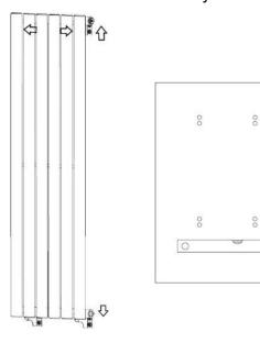
3. Using the drill and 8mm drill bit, drill into the marked positions then insert the wall plugs and tap flush to the finished wall surface.
